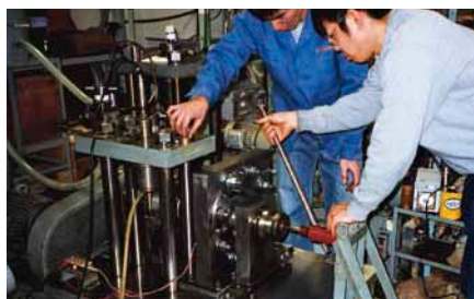
内歯車の曲げ疲労試験の準備 Preparation of bending fatigue test of internal gear by students
